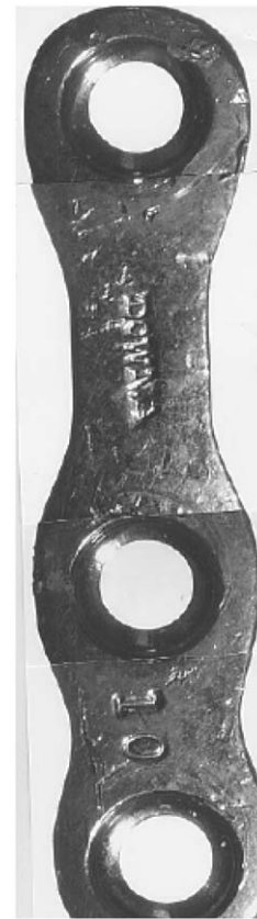
Figure 3 Close-up of the removed plate, showing that no corrosion appeared on the plate. The manufacturer's name "DOWN.A" was still clearly readable.
